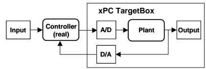
• Limited deployment — Using stand-alone mode, connect an xPC TargetBox to your plant, and run the control software without a connection to a host PC.
