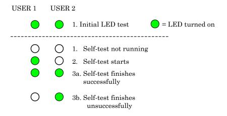
**10** Observe the sequence of LEDs turning on and off.
