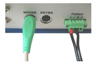
2 Use a keyboard with a PS/2 connector and attach it to the back panel of your xPC TargetBox.
